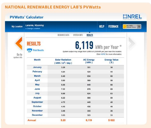
PVWatts is the most commonly used tool for evaluating solar resource. Novices and experts can use the easy-to-use platform. PVWatts even allows customized sizing of a solar array and variations based upon slope and orientation. The tool also offers rudimentary financial analysis. http://pvwatts.nrel.gov
