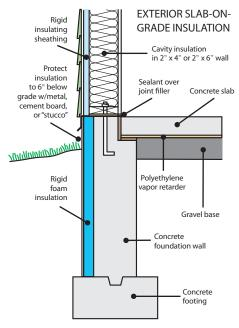
Foam boards are the most common form of exterior slab-on-grade insulation. The above grade portion must have UV and structural protection.
