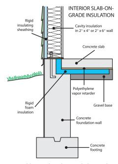
Interior slab-on-grade insulation can be horizontal. Interior placement avoids the need for protection, but may require cutting small pieces and more difficult details.
